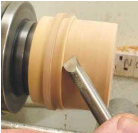
STEP 19. Once the apple is mounted up on the jam chuck, turn it down to fit inside the rosewood base. The little shoulder will be the part of the light timber that will be seen from the outside
